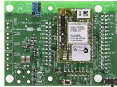
(c) DC9018: External antenna mote (2 deployed)
